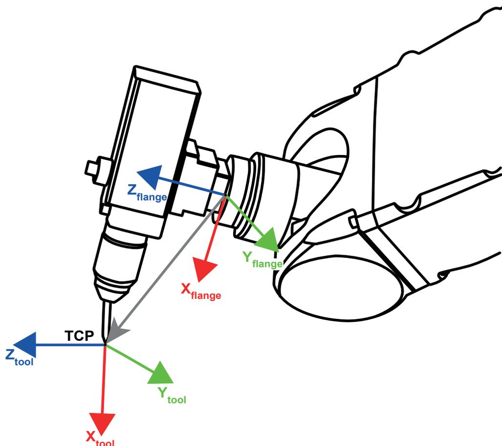
Figure 1: Tool coordinate system (TCP) relative to the robot's flange coordinate system
