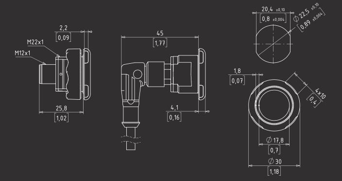
All dimensions in mm. Imperial measurements in square brackets
